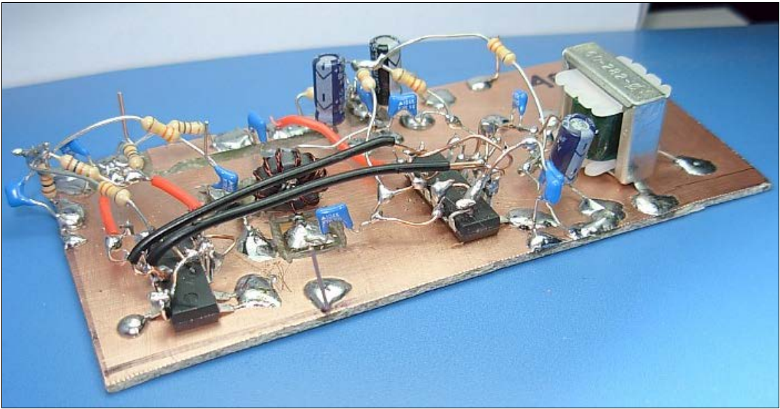
The breadboard of the 4066 Concept schematic shown above.
