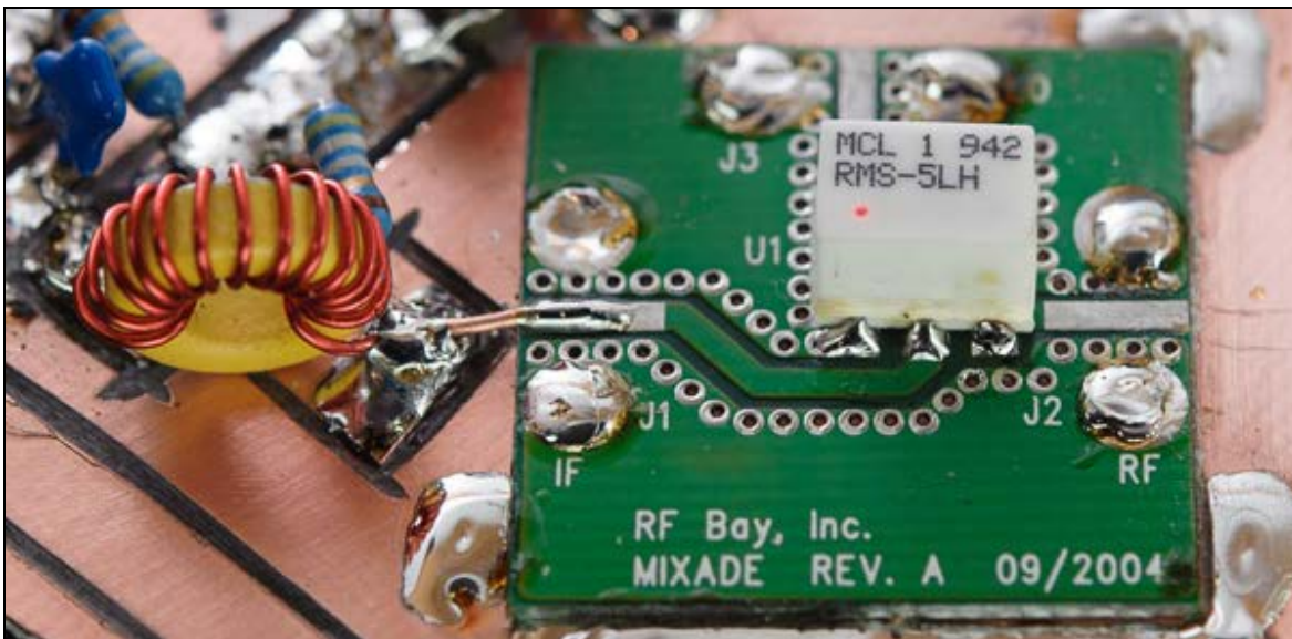
Above — Mixer and diplexer assembly. The RMS-5LH takes 10 dBm LO drive.
