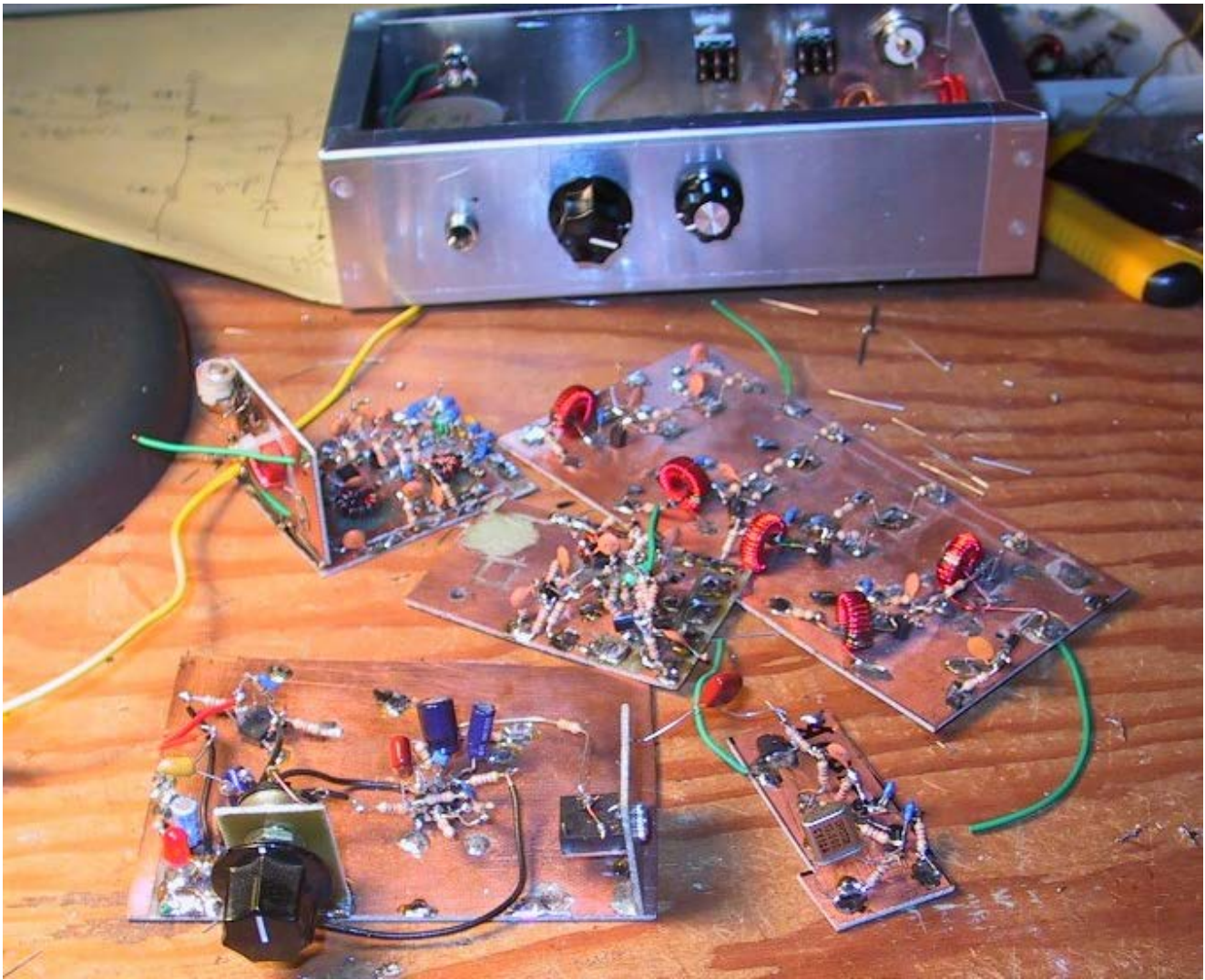
Above graphic. Some of the bread boards developed during experimentation. My final receiver layout (and potentiometer positioning) is not optimal, however this is a prototype and I had no idea what the finished version would look like.
