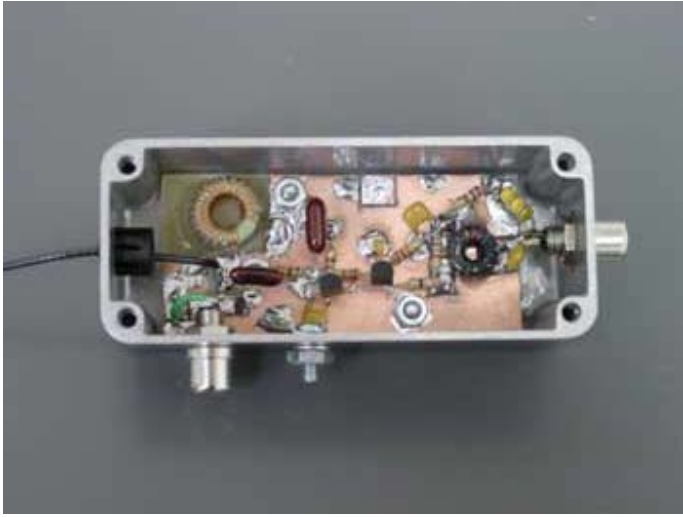
Above left: Inside Joe's trunk lid SWL Active antenna. Great ugly construction in a sturdy Hammond chassis. Above right: Joe's remotely tuned SWL active (or voltage probe) antenna amp and whip holder. Thanks Joe!
