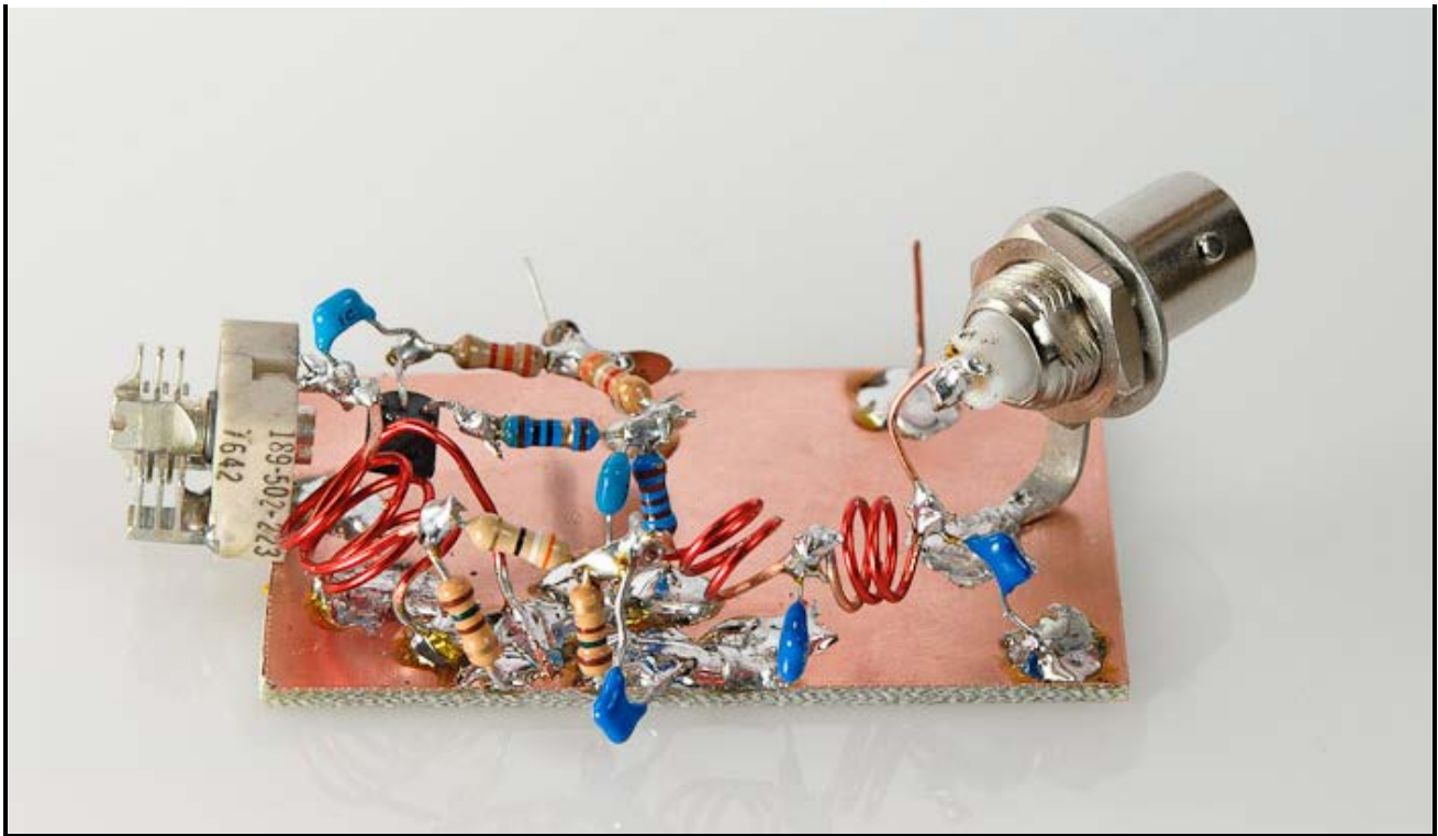
Above — I built a prototype 200 MHz oscillator with trailing low-pass filter before making the 210 MHz version placed in the 1-118 MHz VFO for the K3NHI sweep system. (Section 1). The secondary coil floats and may be positioned between any of the 4 primary links to change coupling and thus output power.
