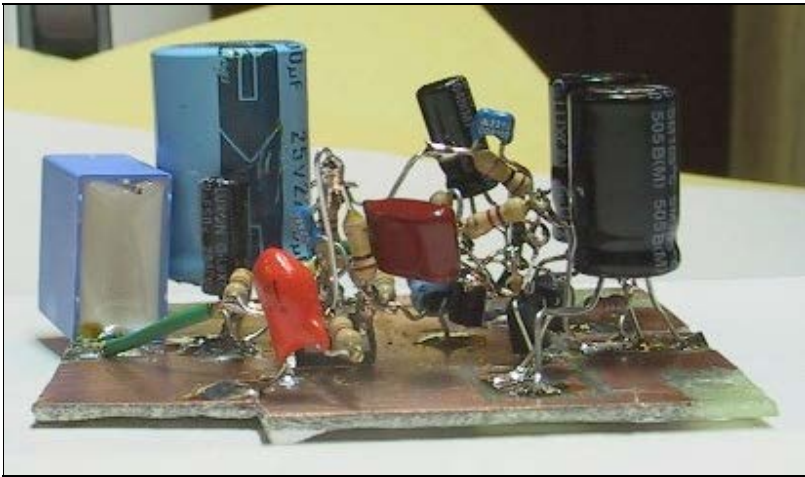
Above, A breadboard of the KK7B audio stage which is preferred to the LM386 stage used in the 5 MHz WWV receiver. The LM386 does take up less room and certainly increases the popcorn factor.
