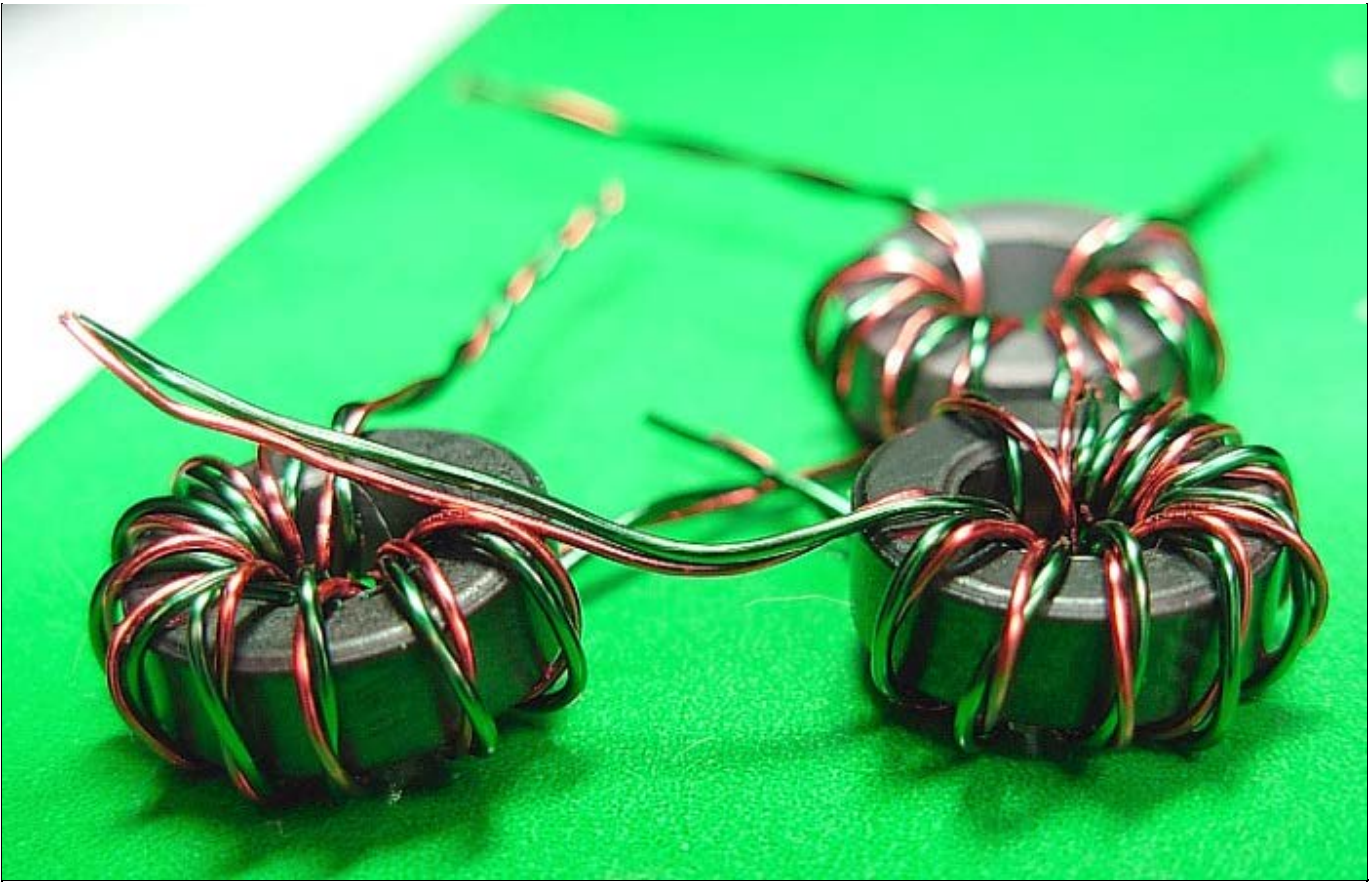
A trio of bifilar transformers wound on FT37-43 ferrite toroids. 2 colors of wire reduces errors and speeds up construction. Consider making up 5 at a time, so you have them on hand and do not have to interrupt your experiments.
