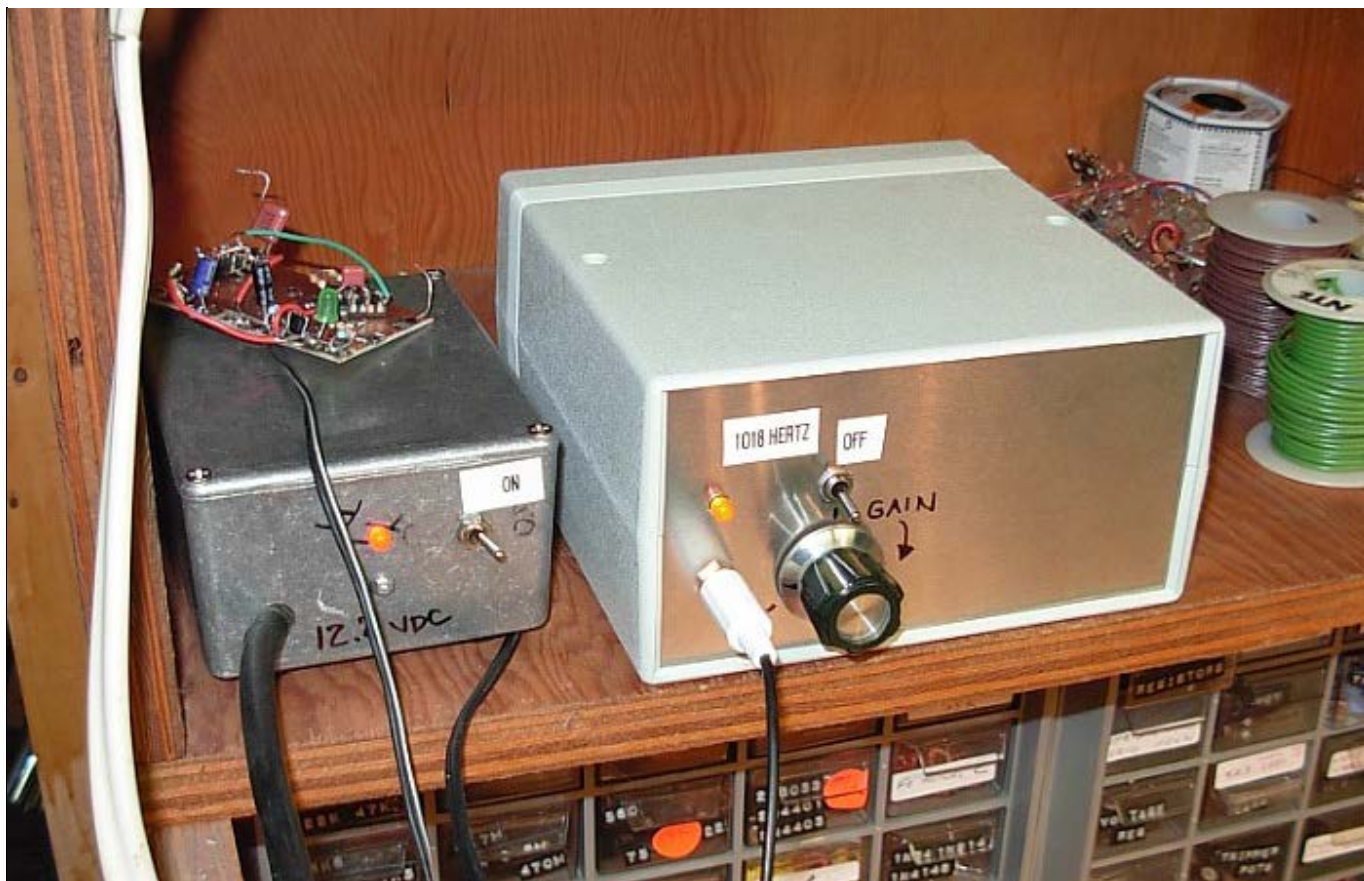
The 12.24 volt DC supply and the 1018 Hz AF audio oscillator used in these experiments.
