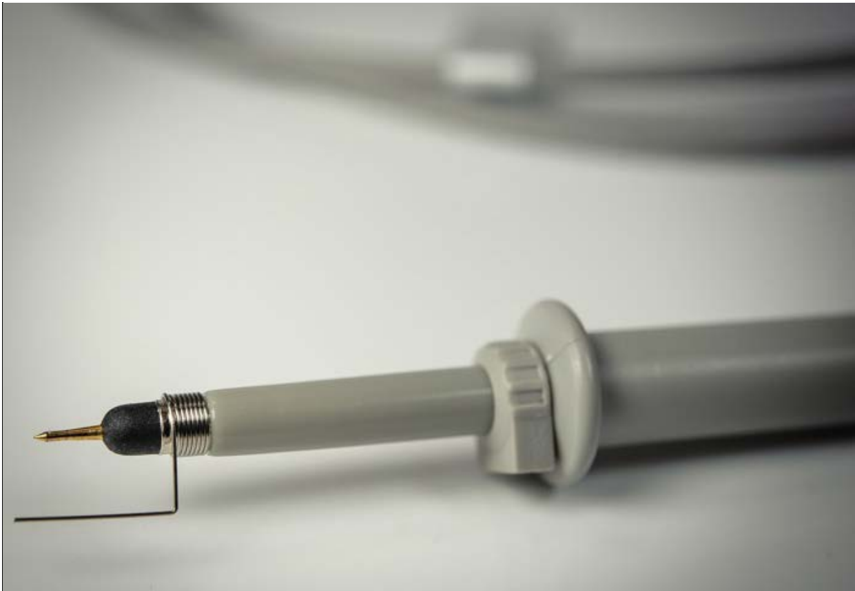
Above — A short 10X probe ground lead boosts Tx measurement accuracy; in particular, for FFT analysis with your DSO. You can read or see why by searching the web for text and/or videos concerning oscilloscope probes.
