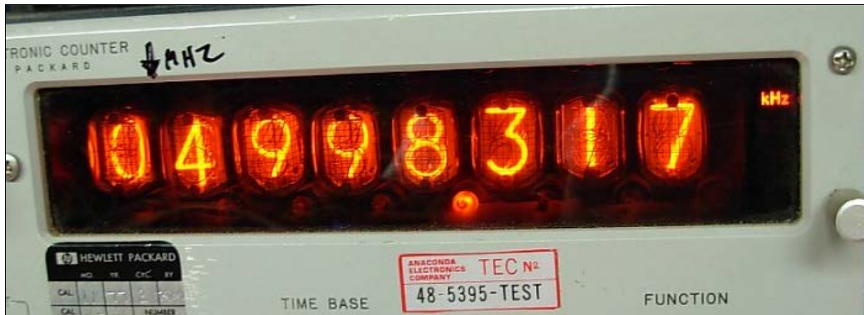
Frequency measured with the switch thrown = 4.998317 MHz
