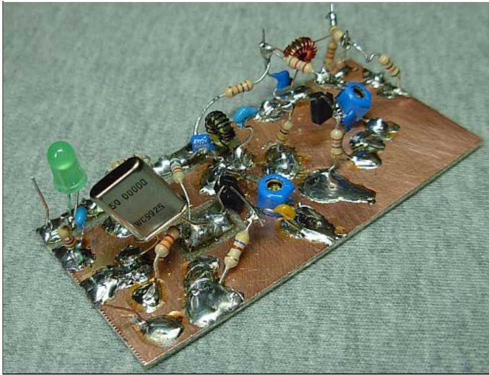
The breadboard of the 50 MHz oscillator prototype.
