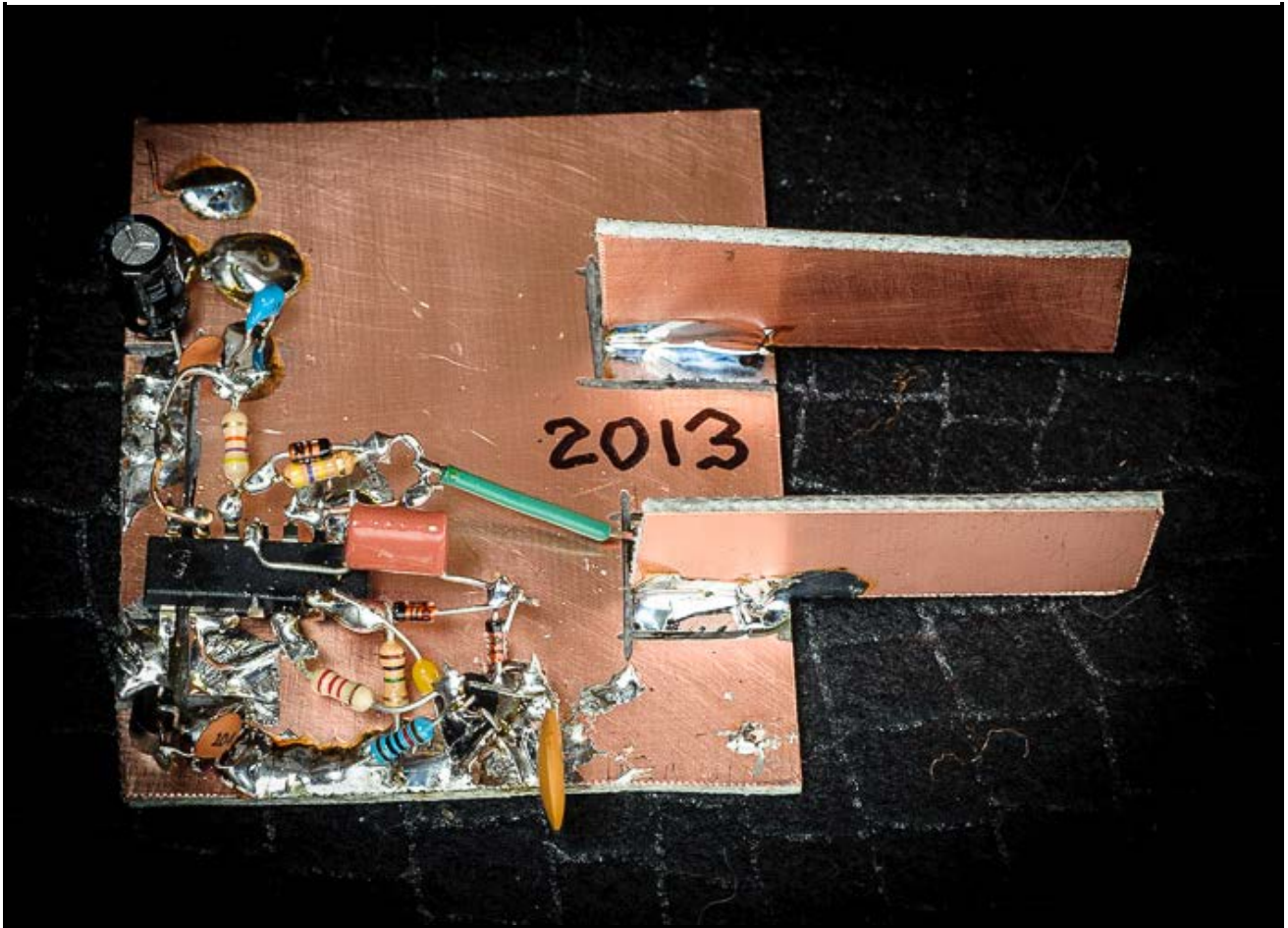
Above — The very ugly development proto-board of my half-done non-mechanical Iambic paddle. At some point I'll build the other half (the dah paddle switch) and press it into service. You might also use this circuit as a non-mechanical straight key.
