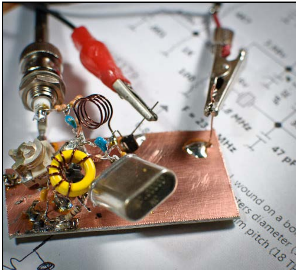
Above — The 5th overtone Butler with an inductor in parallel with the crystal
