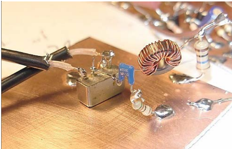
A diode ring mixer was used as a reference mixer in the product detector experiments.
