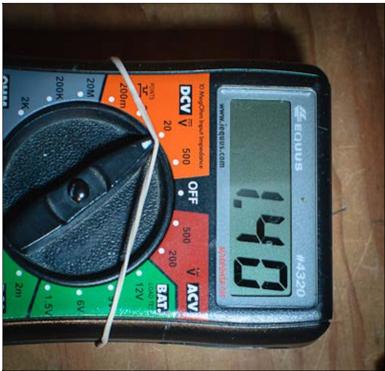
Above — The Port B voltage when a 10 dB attenuator pad was connected to the calibrated -10 dBm sine wave signal source: Measured power = -20 dBm. Notice the 20 mV/dB power drop — right on specification.
