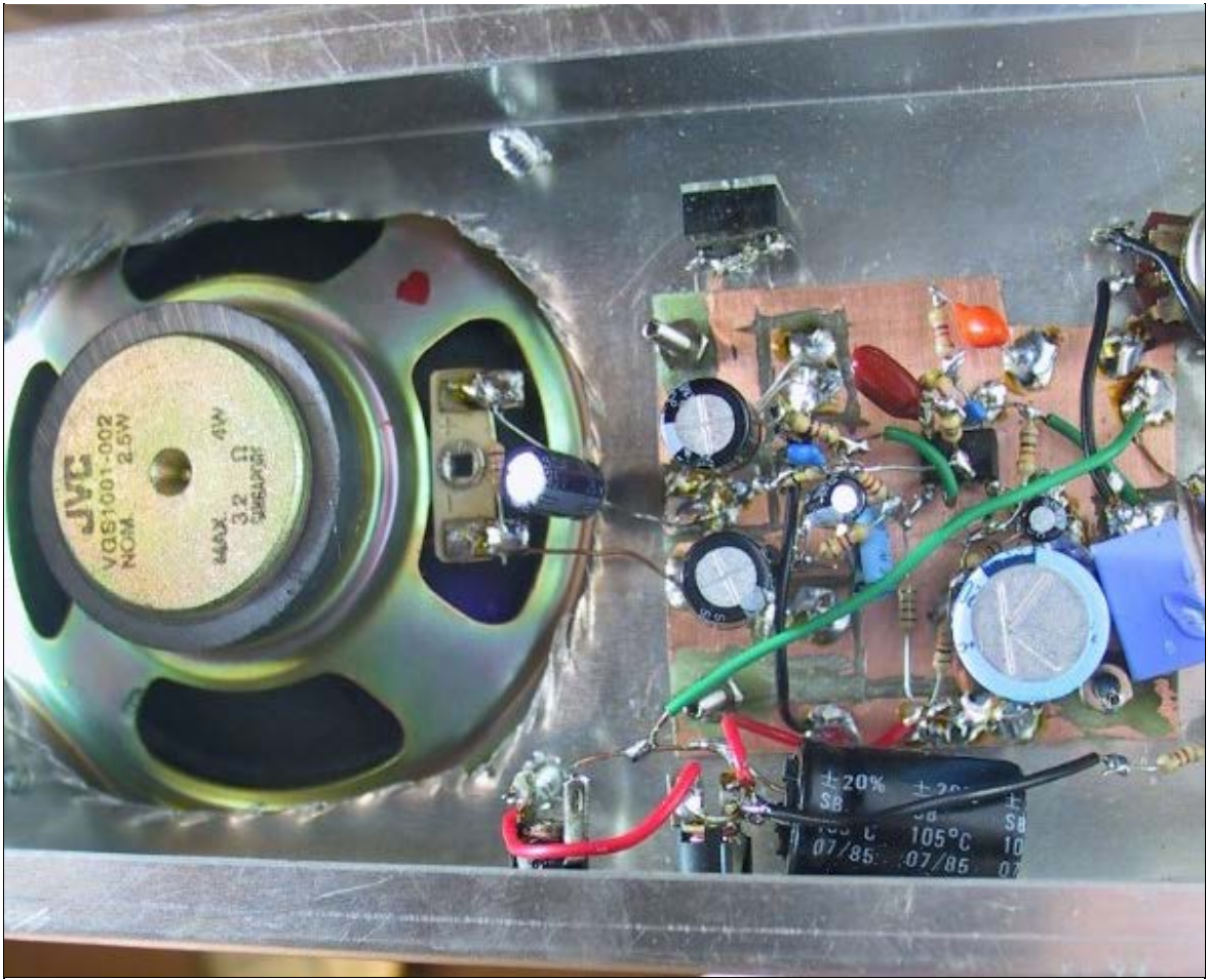
Above. The AF stage shown above in a chassis containing a speaker. This is my lab AF amp for testing receivers on my work bench.
