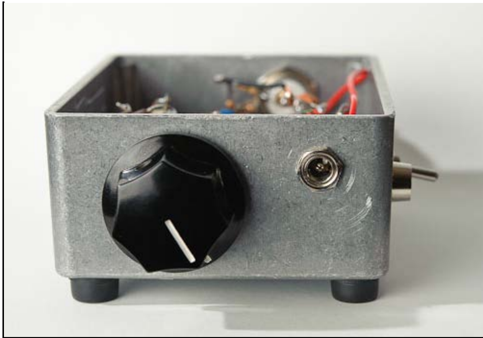
Above — A 7 MHz Vackar VFO with the lid off
