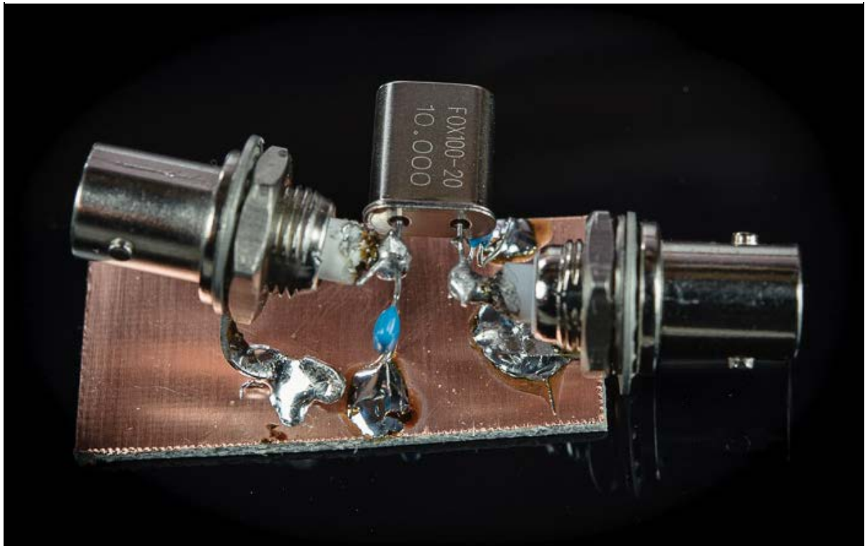
Above — 10 MHz Crystal filter breadboard.
