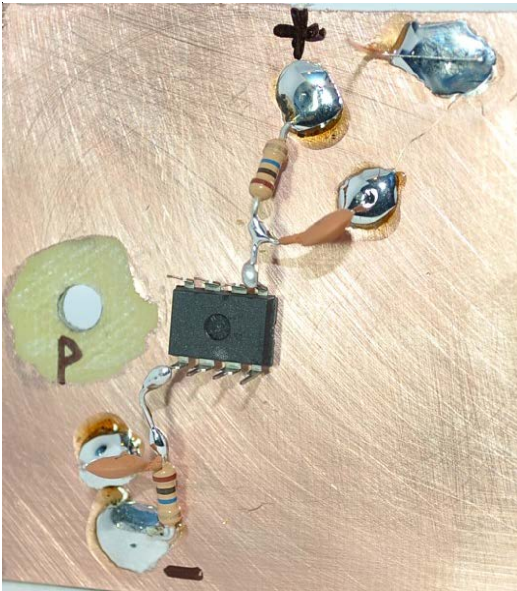
Above — a method to anchor op-amps using a split (negative and positive) power supply. Pins 4 and 8 are soldered to the copper board via a 10 megohm resistor. A 0.1 uF ceramic bypass capacitor is also connected to these pins. The resistor leads were left a little long to allow easy connection of the power supply wires. I write each pin's polarity on the board to avoid wiring mistakes.
