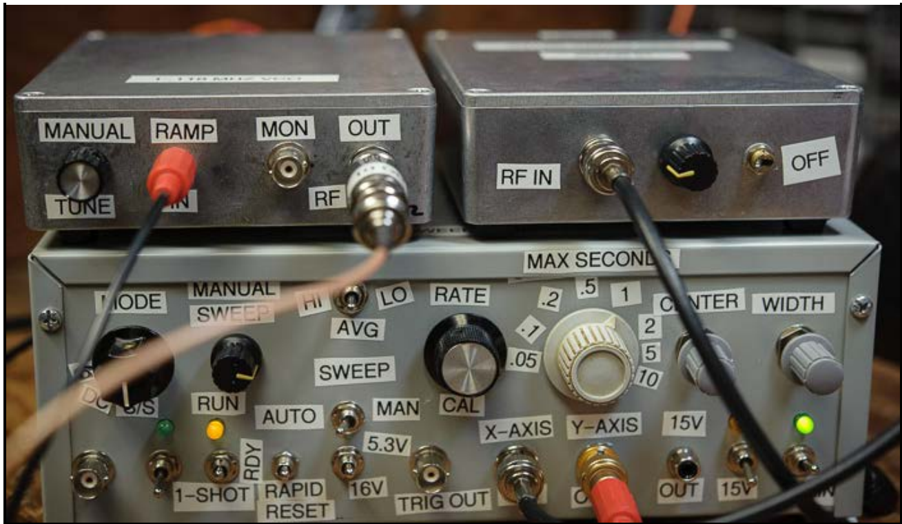
Above — The K3NHI sweep system in action. This photo shows the power meter with the (later) added DC offset control. Using the offset control potentiometer, I'm able to examine the top of a signal peak at 1 dB per division with various spans.
