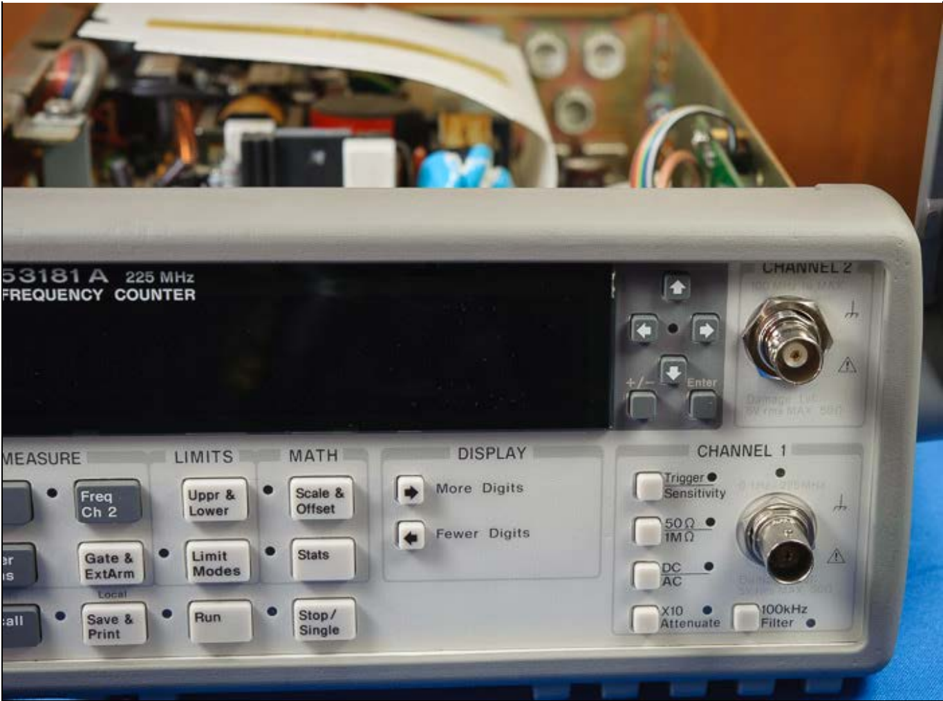
Above — My HP counter with the kit installed as Channel 2.
