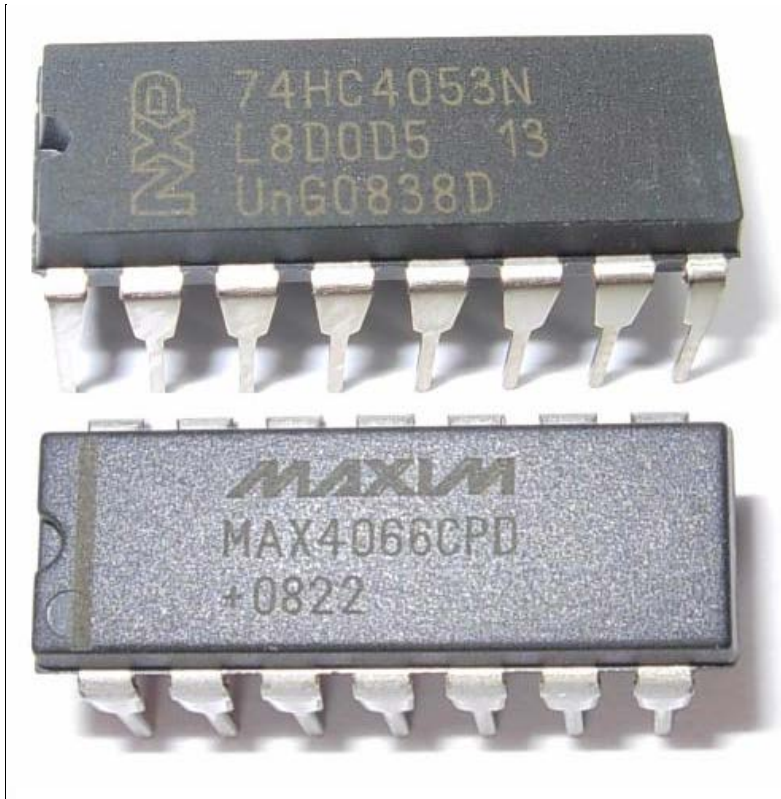
The DIP IC switches used as product detectors in the K7LR memorial receiver experiments.
