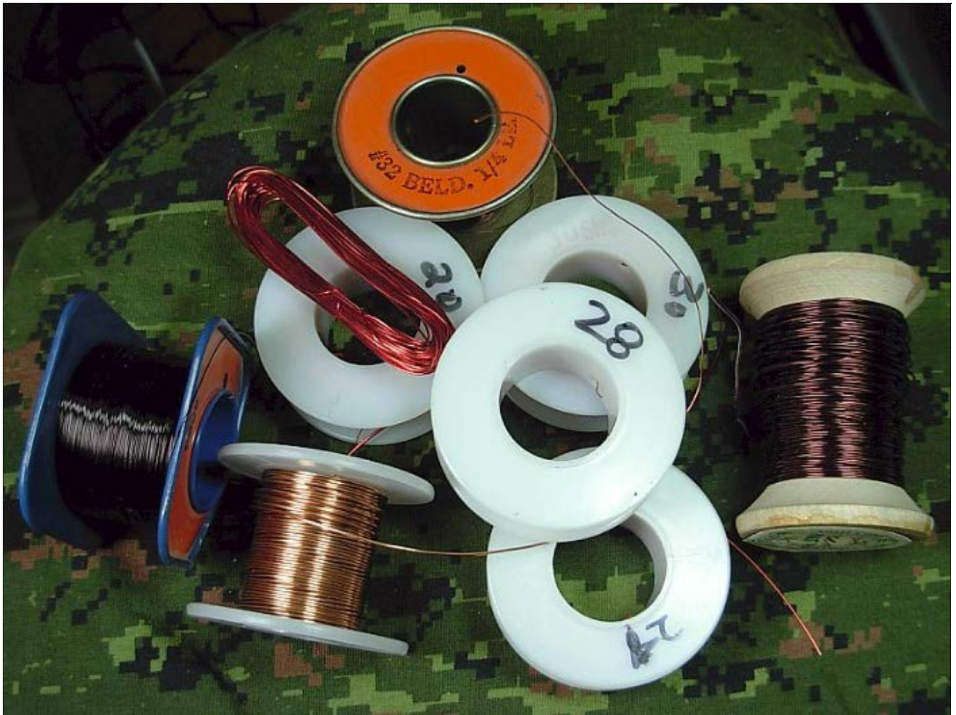
A sample of the enamel coated copper wire collection I wind inductors and transformers with. In stock are wire gauges from 18 to 34. Like everything else, this collection started small and grew over time. Be vigilant for bargains and when you find a good price, purchase a whole bunch as it does not go bad. The Belden wire (orange spool ends) is over 40 years old and the enamel insulation remains perfect.
