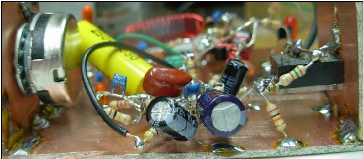
Close up of the KK7B audio amplifier breadboard from the 10K potentiometer to headphone jack
