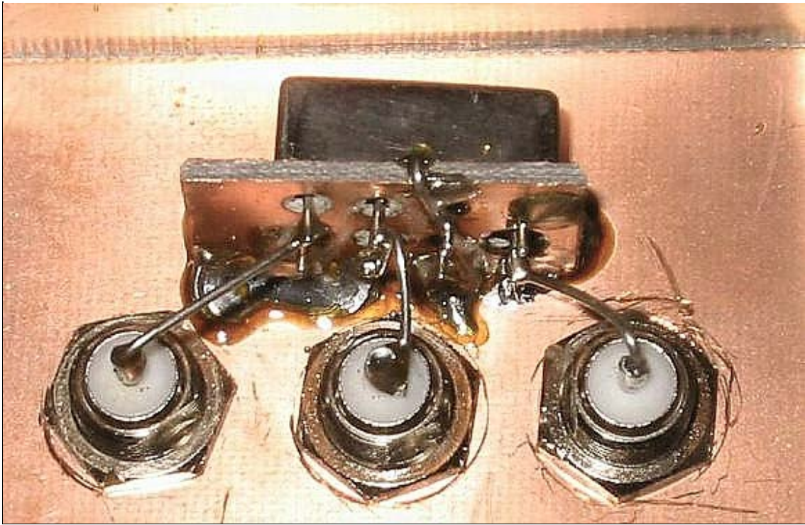
Figure 2. The inside of the module containing a Mini-Circuits SBL-1 diode ring mixer. This is a standard part that is essentially generic. The first experiment was to set up a pair of 10 MHz signal sources. One was from a homebrew generator, shown below.
