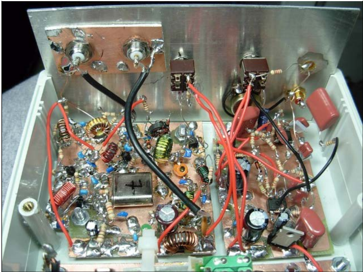
The 7 and 14 MHz crystal oscillator board mounted in a project chassis along with a 1 kHz low noise oscillator. This photo was a prototype version that did not have a Chebyshev low-pass filter after the 14 MHz stage.
