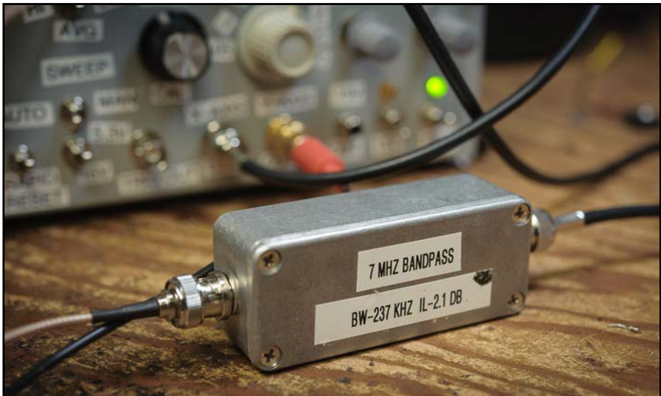
Above — I swept a 7 MHz band-pass filter bench module.
