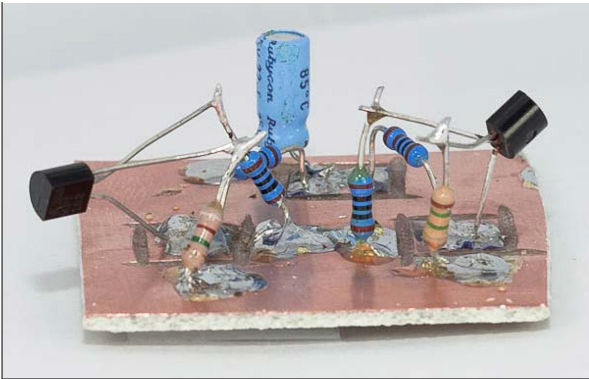
Above — A differential FET matcher breadboard. This version had a 9.1M gate resistor on Q1 by accident, although it made no difference to the experiment, as no DC gate current flows.
