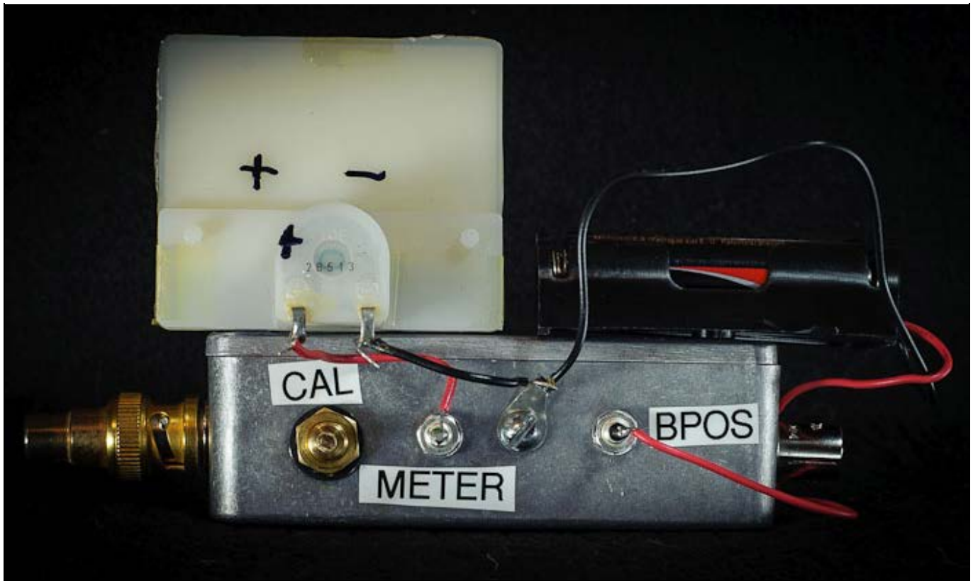
Above — My prototype RF-tight breadboard of the Barebones PM. I ran my 'trademark' die case box, BNC RF input and Port B connectors, a common ground lug and feedthrough capacitors for the B+ and panel meter connections. I placed a BNC to RCA adaptor on Port B to allow the insertion of a standard-type positive DVM probe. A black alligator clip terminates the distal end of the negative probe on all my DVMs. I just clip it onto the ground lug.
