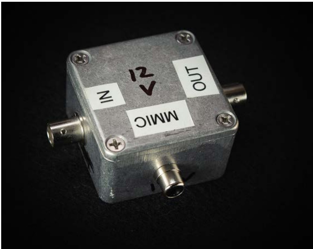
Above — The completed amplifier module in a Hammond box with an RCA jack for the DC voltage.
