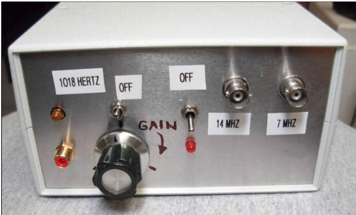
Front view of the .001, 7 & 14 MHz oscillator. It is really fun to build your own test equipment.
