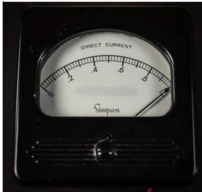
Above — An antique 1 mA panel meter driven with 1 mA to achieve full deflection.
