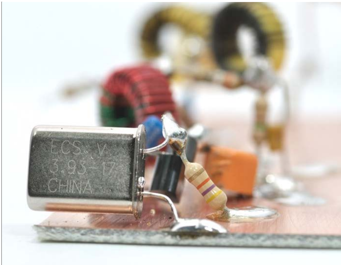
Above —The LO breadboard in close-up using a long focal length lens. Click for a wide angle photograph. The unsoldered end of the 100 \Omega resistor in the close up photograph is where I connected the VCC.
