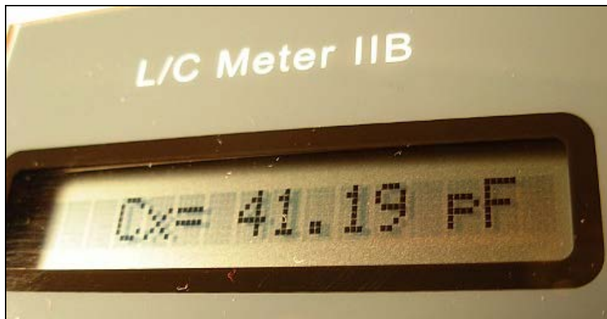
Parallel capacitance of the above 5.0 MHz crystal in an AADE LC meter
