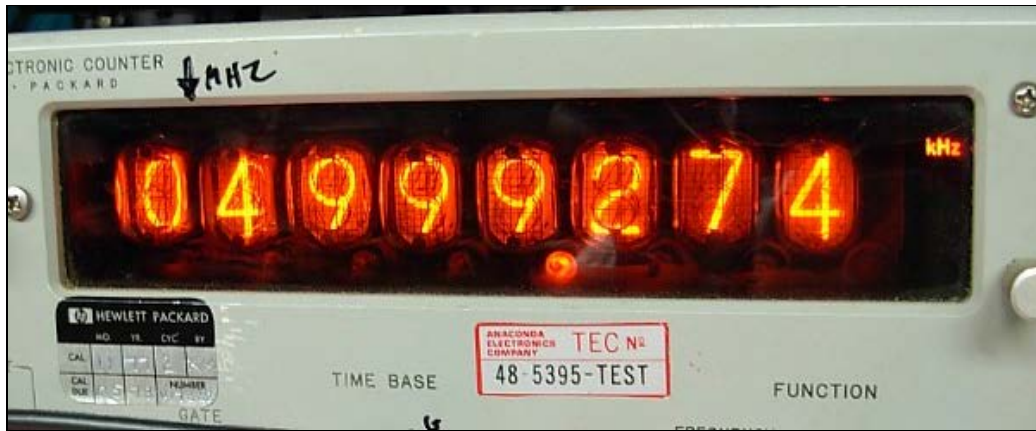
Frequency measured with the switch open = 4.999274 MHz
