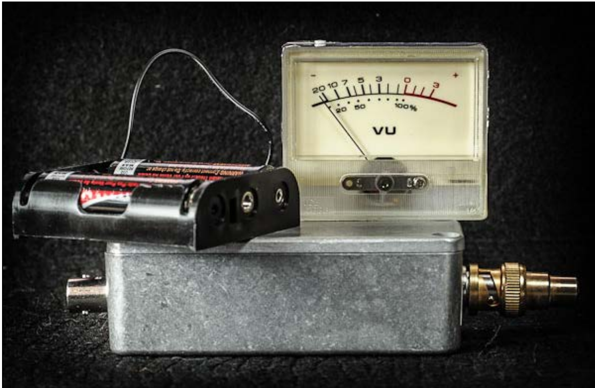
Above — A view of my breadboard showing my 100 uA panel meter and the 4.5v battery pack. I raised R2 in the original schematic up to 8K2 to set my preferred needle movement in this 100 uA panel meter. A meter with linear markings might be better?
