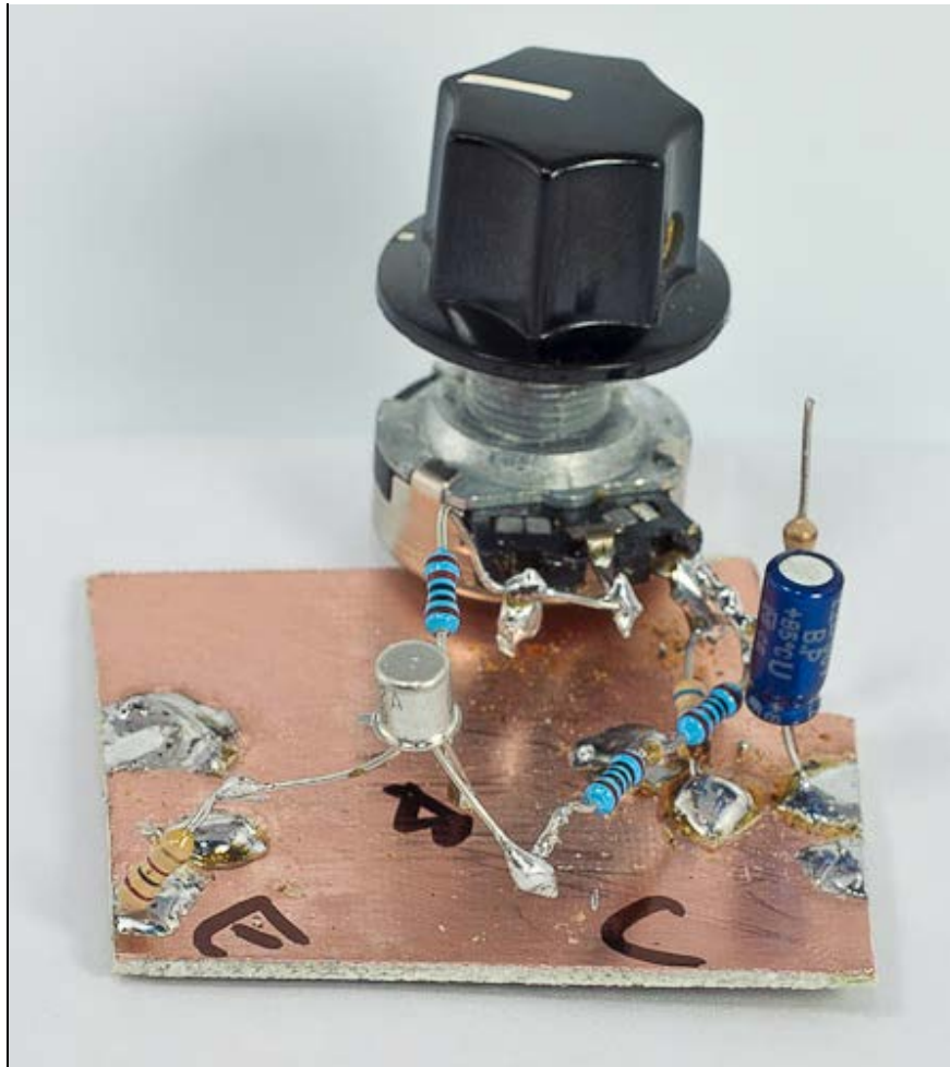
Above — Breadboard of the QRP beta tester. We hope you have as much fun with this circuit as we did.
