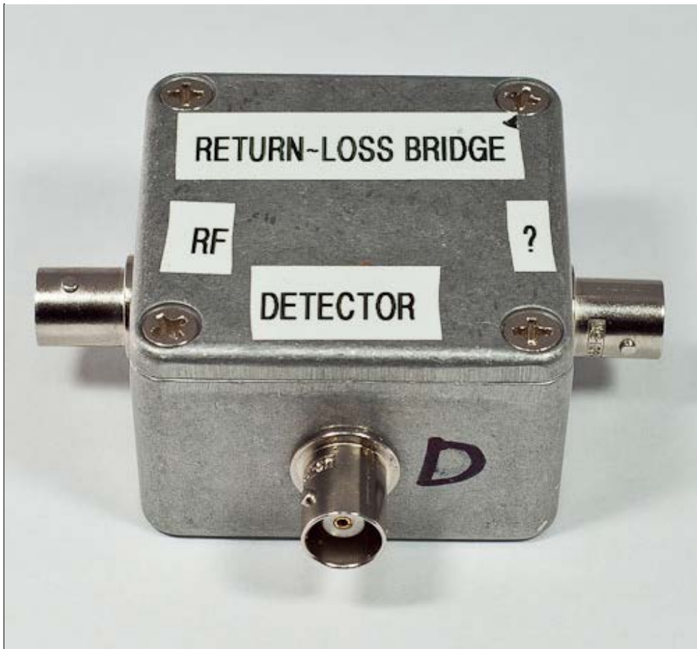
Above — The completed RF-tight bridge. Don't forget to label your network ports.
