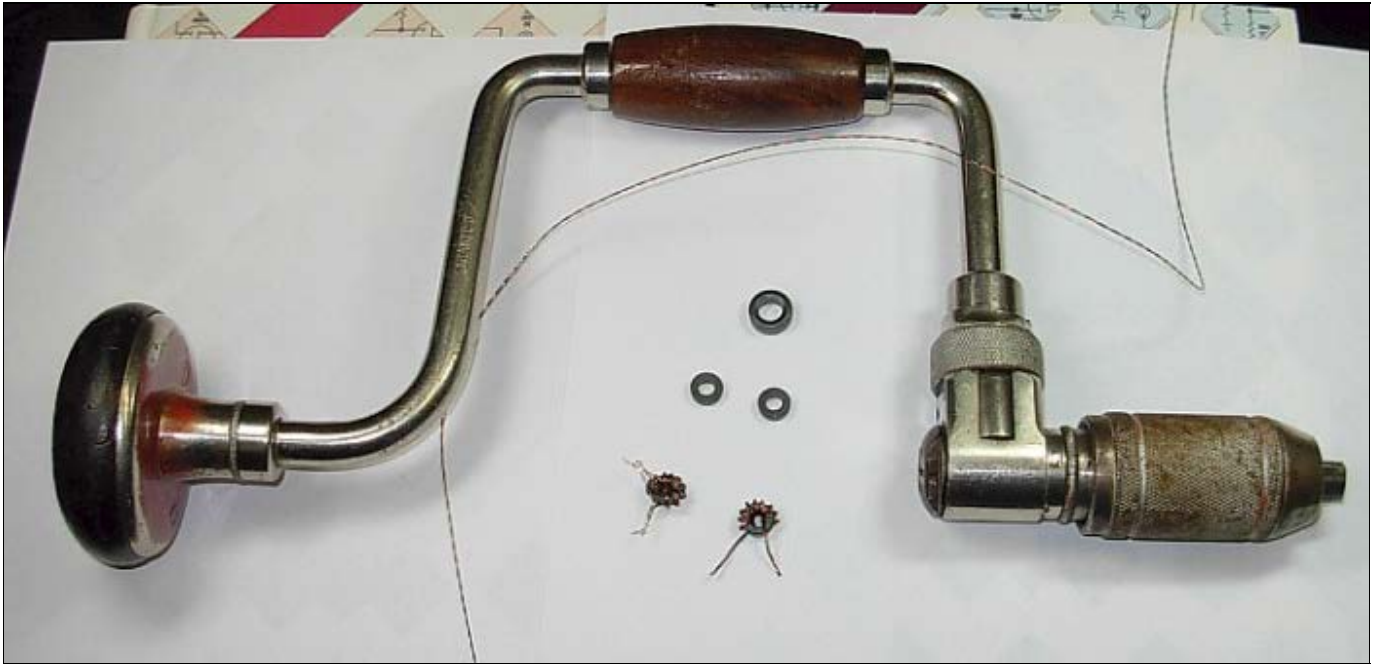
A brace and bit hand drill plus a vise provides a good way to twist your wires.
