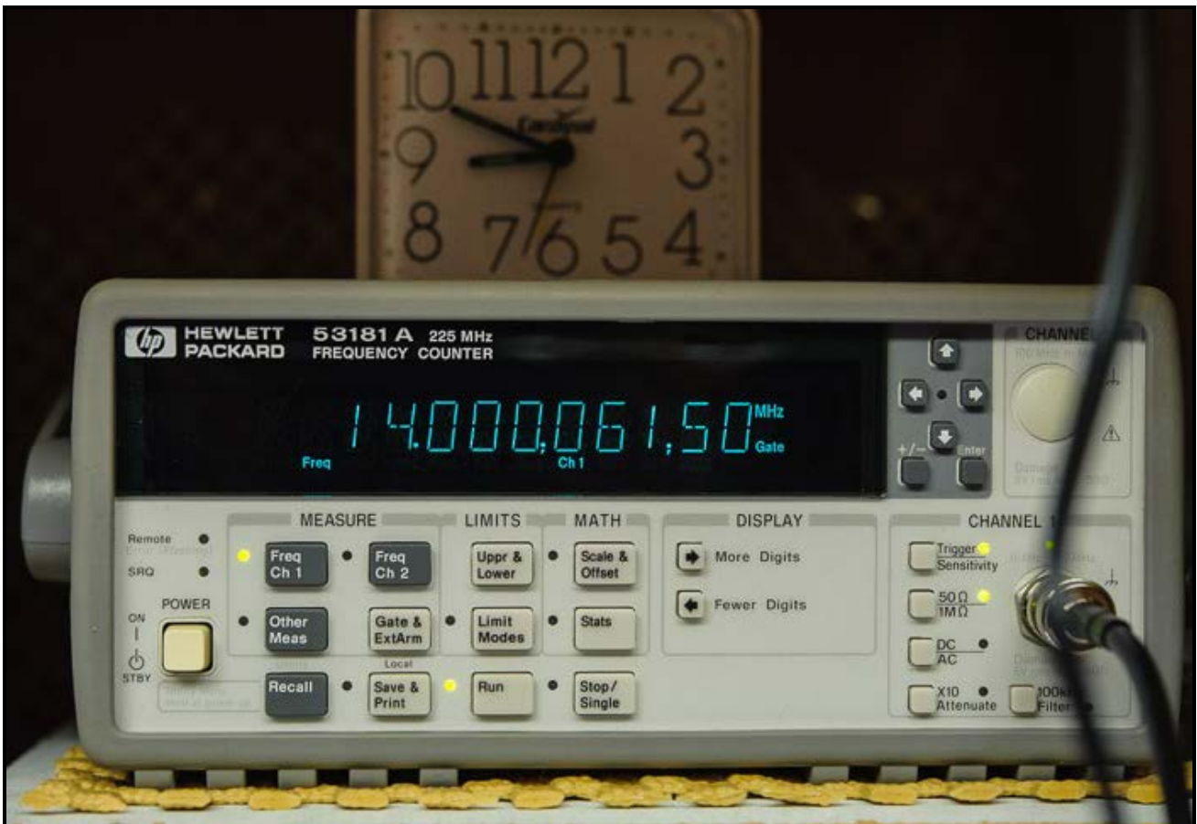
Above — My VCO frequency with the 1.5 MHz MTO set at full mesh. Since my MTO only tuned from 1.50 to 1.52 MHz, my VCO only tuned from
