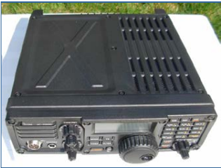
Top angle view. There are ventilation holes at the top right hand side. You can just see the ventilation screen just next to the right top panel screw.
