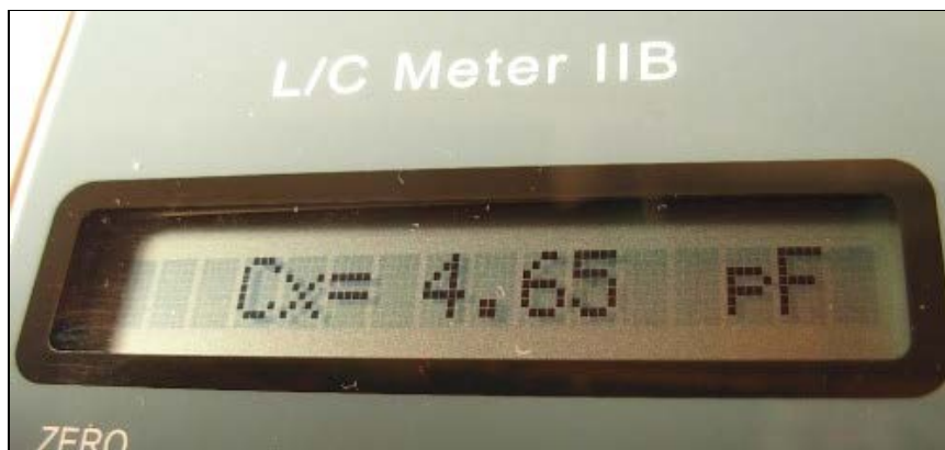
Parallel capacitance of the above 5.0 MHz crystal in an AADE LC meter
