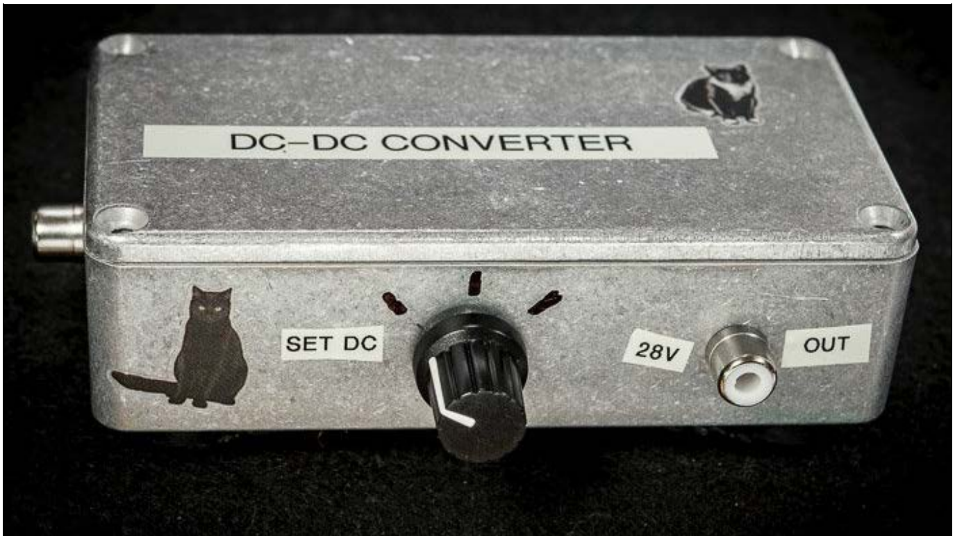
Above — Bench module: 28v DC to DC converter. While containing no tuning control pot, my build places the zener diode regulator control potentiometer on the front panel to allow fast-tweaking of the output voltage from ~21-30 VDC depending on the load. Click for the breadboard photo.
