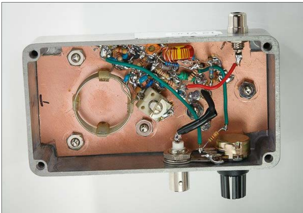
Above — A photo of the completed Colpitts LC oscillator. Running a phono jack for the DC input was a mistake. A feedthrough capacitor = the best choice. The epoxy glued air wound coil and air trimmer cap plus the regular temperature stability techniques and a 100 pF polystyrene
