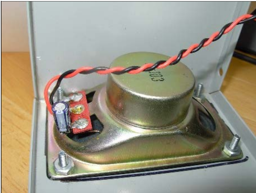
The photograph above shows the speaker attached to the Hammond chassis top. Holes were drilled in the chassis lid with a drill press to allow the sound to pass through.
