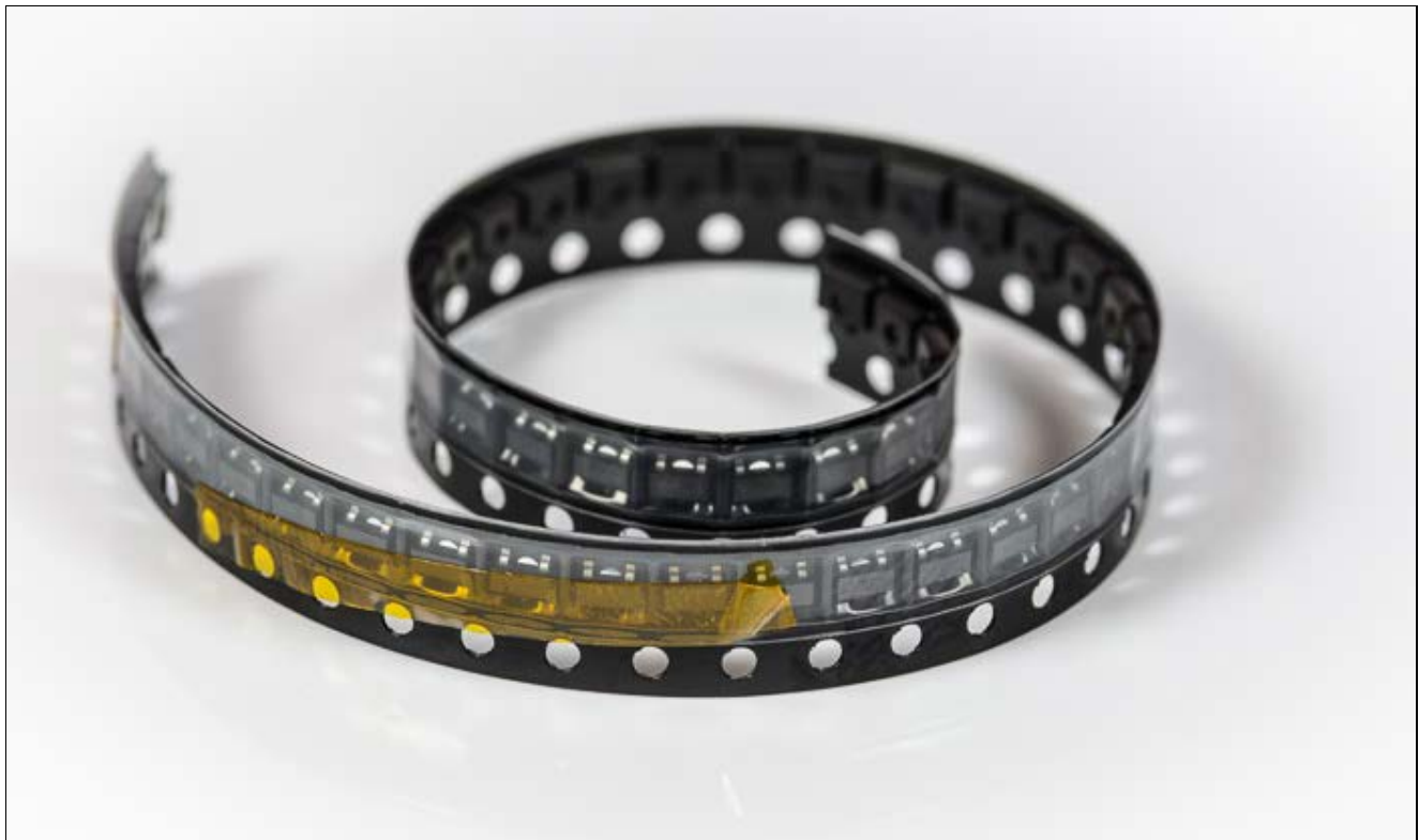
Above — A 5X magnified roll of 50 BFS17A in SOT-23. Compact or what?
